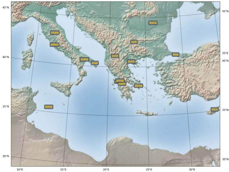
Figure 2.6: Considering a minimum distance of zero kilometers, 16 NTRIP GNSS datagrams are selected in Greece and its surrounding area for their acquisition at 1 Hz.
